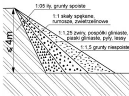
Fig. 1 The inclination of the walls of the trench depending on the type of soil (5)
